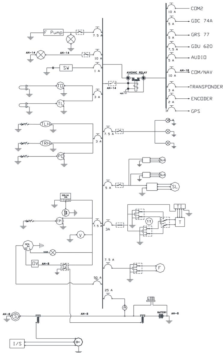
The Garmin G500 units are connected to the avionic bus through dedicated circuit breakers.
