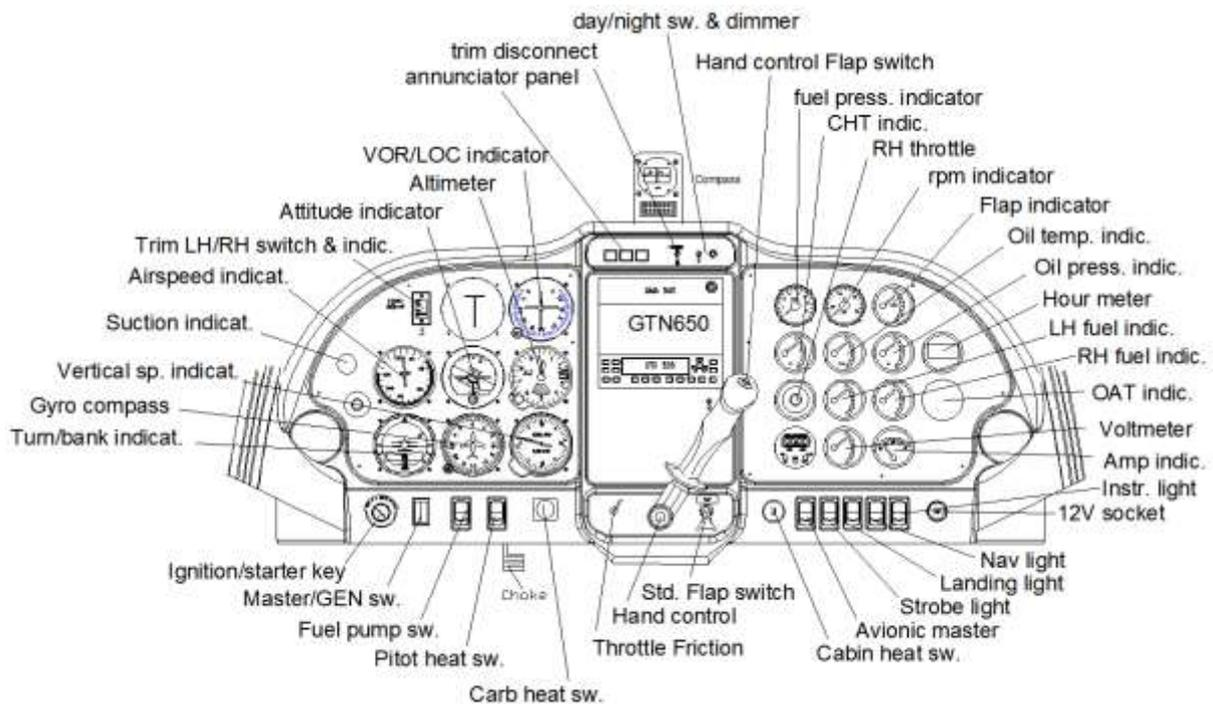
Fig.A14-6. Instrument panel
