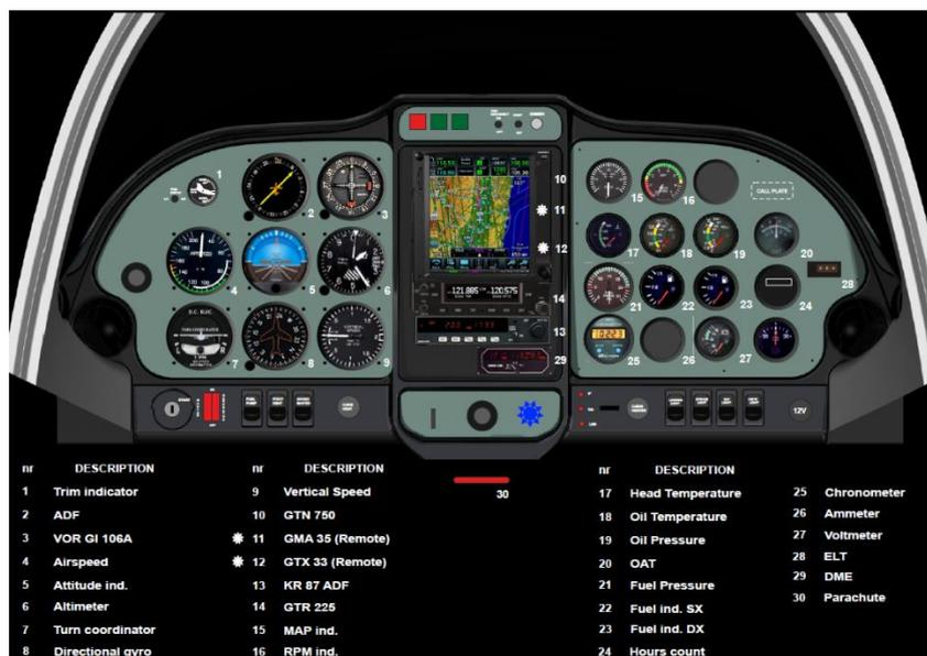
Figure A03-1 NEW ANALOGICAL INSTRUMENTS PANEL (ONLY FOR REFERENCE)
