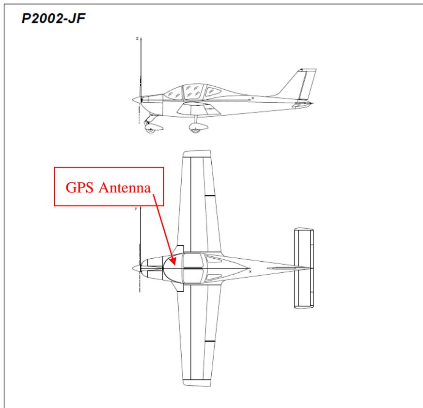
Figure 3 - Position of GPS Antenna-GTX 335 behind cockpit
