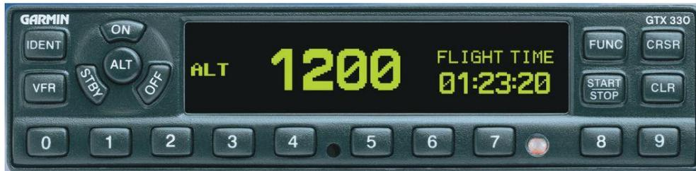
Figure 1 – GARMIN GTX330 Transponder
