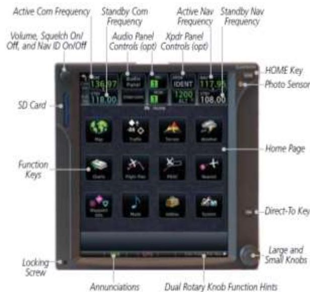
**Figure 1- GTN 750 Control and Display Layout**
