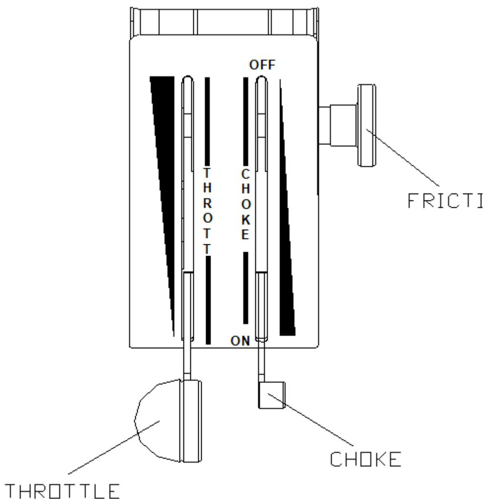
Figure A05-1 Central throttle control system
