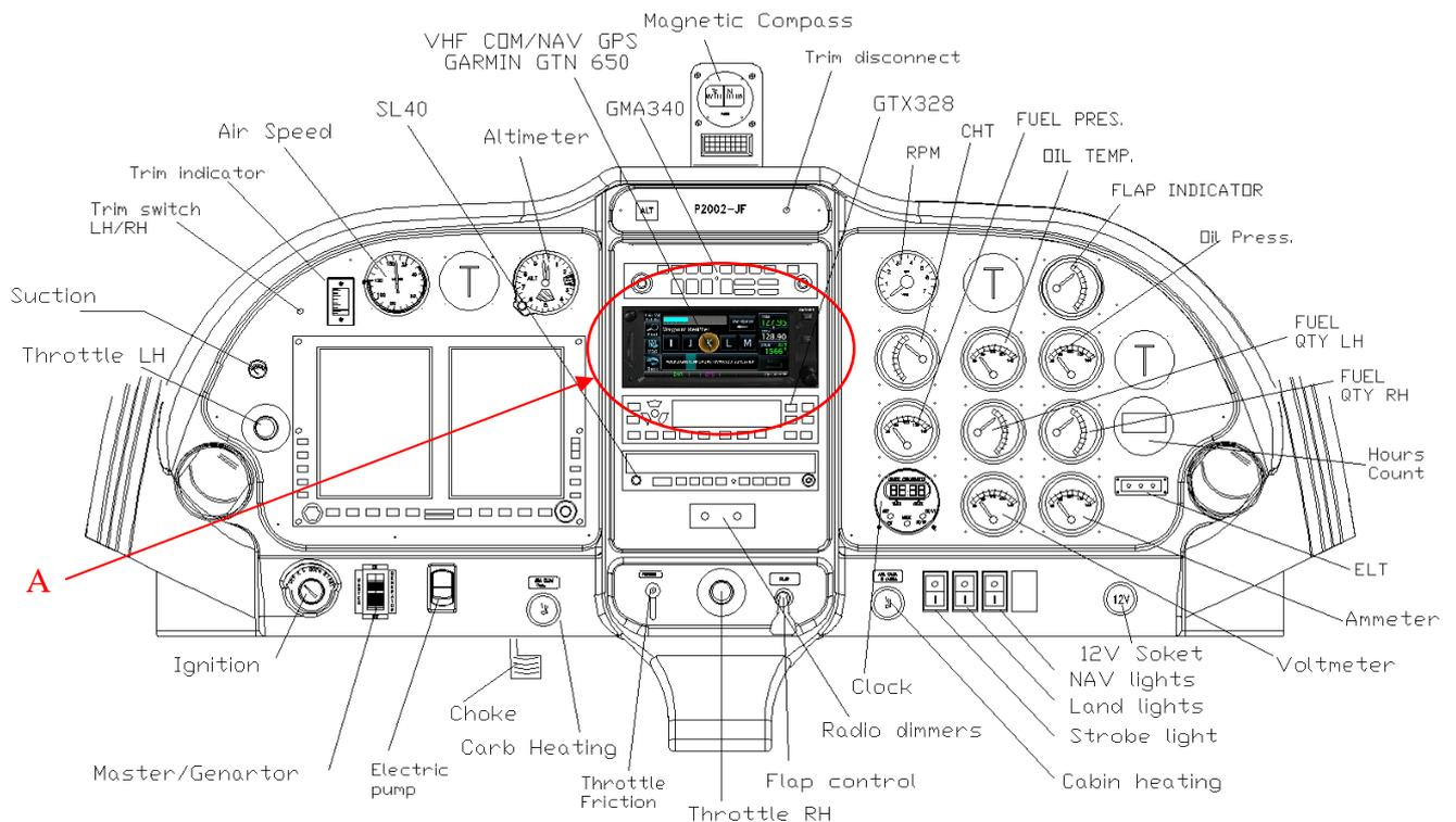
**Figure 1 – Example of cockpit layout of P2002JF with GTN 650/650Xi installation**
